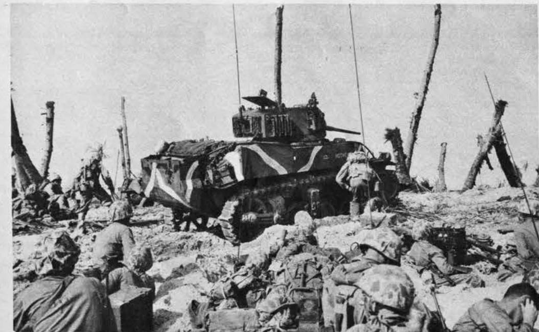
Newest model light tank, M-5A1, moves up on Namur Island, Kwajalein Atoll. Its turret is like the M-5's with the exception of a boxlike extension in the rear which houses the tank's radio.
